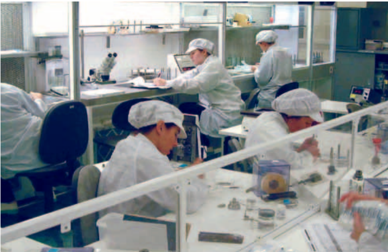
All Barden precision bearings are assembled under stringent cleanroom conditions.
