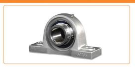
Pillow block bearings, in fact, are variations of deep groove ball bearings. Its characteristic is spherical outer ring surface, It can be equipped to self-aligning capability when it is put inside the bearing housing. Because of low precision and rough structure, pillow block bearings have priority to be used in simple equipment and spare parts, such as agricultural machinery, transportation systems and construction machinery.
