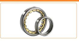
Cylindrical roller bearing belongs to separable bearing. Cylindrical rollers and raceway are line contact with low friction and high speed, can accommodate relatively heavy radial loads. This type of bearing contains Single, double and multi-row bearings, full complement bearings (without a cage) and split bearings. Used in large and medium-sized motor, locomotives, machine tool spindle, gas turbines, reducer, vibrating screen and lifting transportation machinery, etc.
