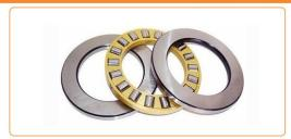
Thrust roller bearings can accommodate combined loads, i.e. simultaneously acting axial and radial loads, but radial loads should not exceed 55% of axial loads. This type of bearing have low friction factor, high speed, and self-aligning. Mainly used in Heavy duty machine tools. High-power Marine gearbox. Oil drilling machine. Vertical machine and other machinery.
